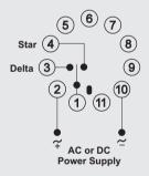
Note: Relay de-energises to the "centre OFF" position when power is off.
